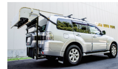
Vehicle fitted with road surface inspection system
