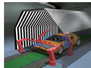
Vehicle exterior inspection example
